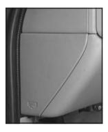
The fuse block access door is on the driver's side edge of the instrument panel. Pull off the cover to access the fuse block.
